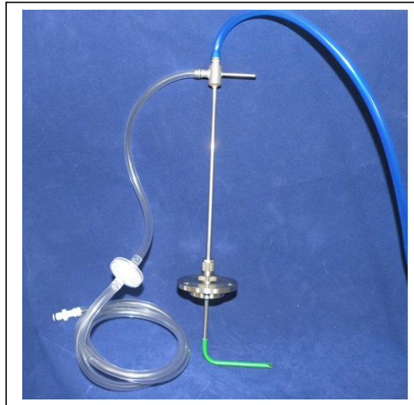
Example of a pitot tube
